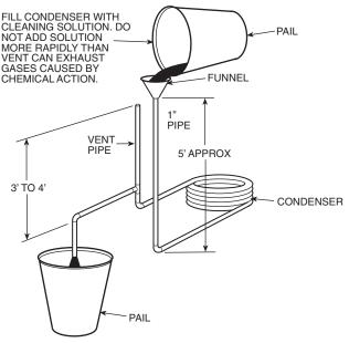
Fig. 37 — Gravity Flow Method
